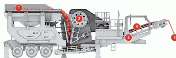
1. Vibrating feeder 2. Jaw crusher 3. Heavy duty rock 4. Discharging belt conveyor
